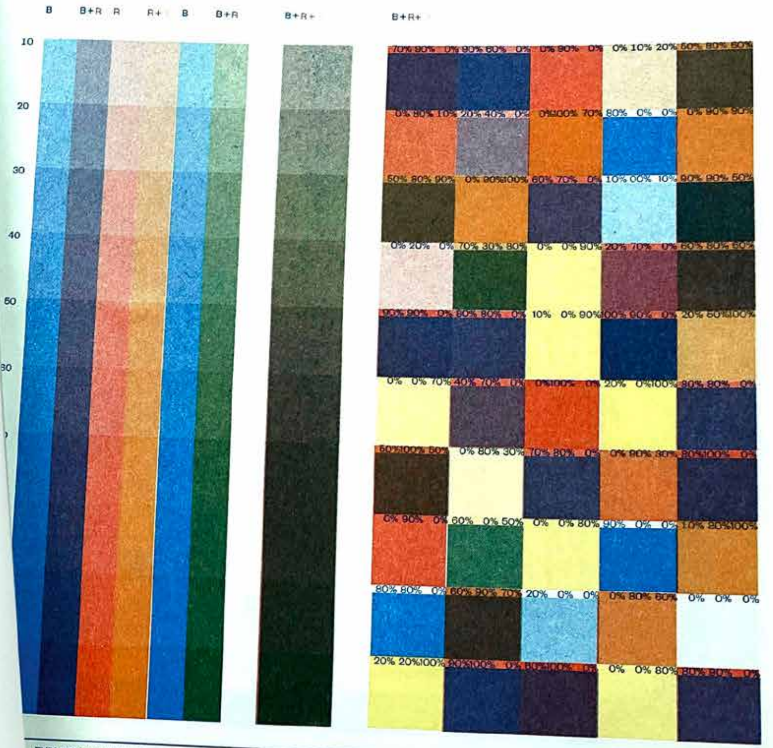
EXPLORISO COLOUR SUITE 1 COLOUR AND SEPARATIONS, 120LPI B (45°) YELLOW R (75°) BLUE YELLOW RED
